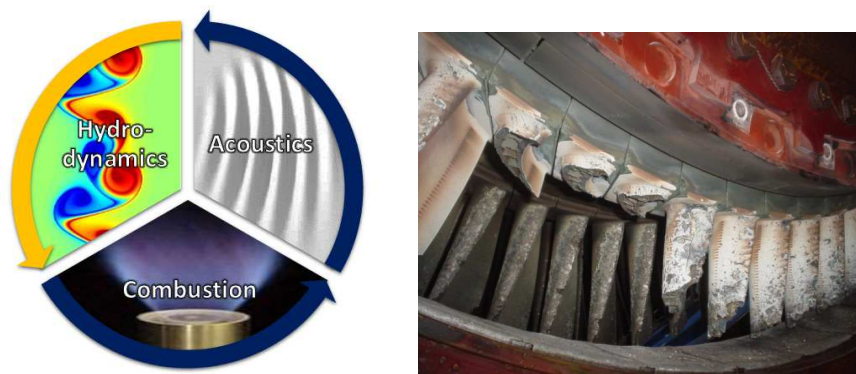
Figure 1.3. Schematic depicting the combustion instability feedback loop (left) and an image of gas turbine blade damage due to combustion instabilities (right).
